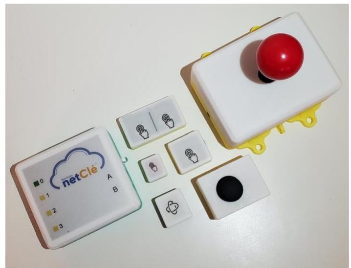
Pictured (left to right): netClé hub, dual touch sensor, mini touch sensor, standard touch sensor, gyroscope, mini joystick, large joystick.
