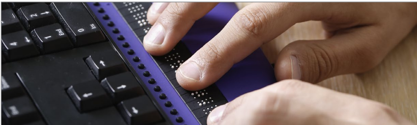
↑ Refreshable Braille Display. A braille terminal with an integrated keyboard and customizable navigation controls. © ZLIKOVEC | DREAMSTIME
